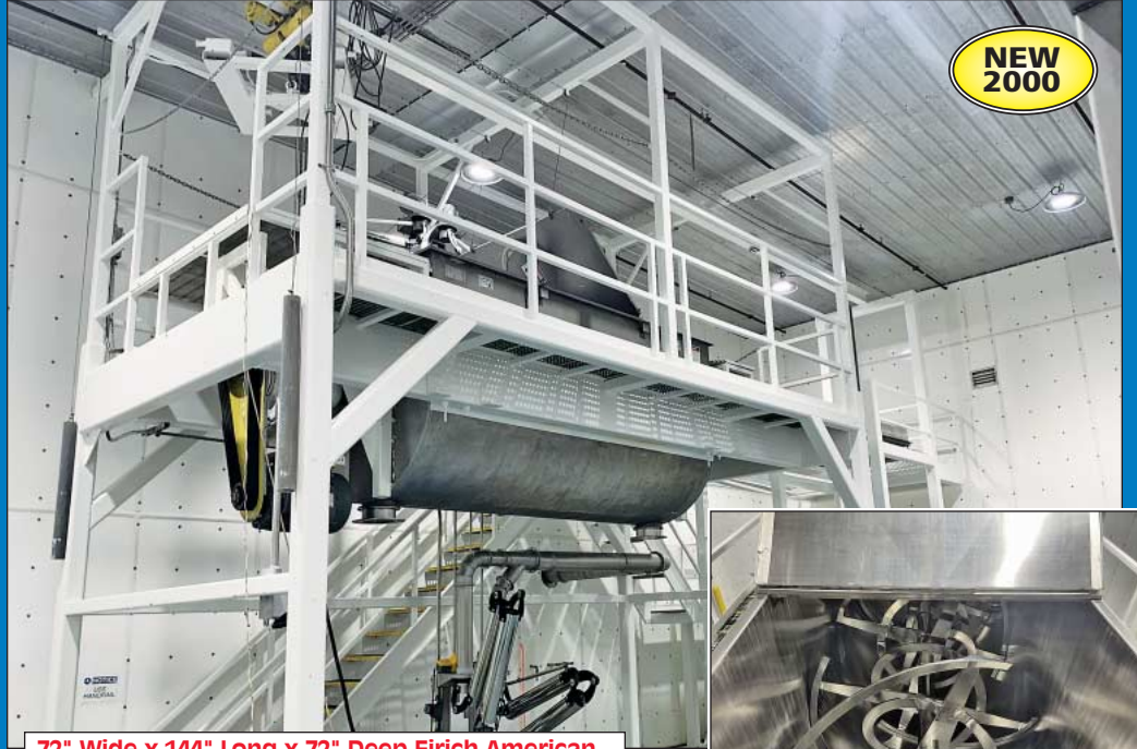
72" Wide x 144" Long x 72" Deep Eirich American Process Systems Model U100/5188 Stainless Steel Ribbon Blender
