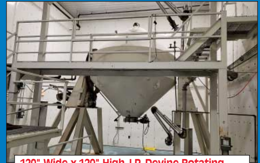
120" Wide x 120" High J.P. Devine Rotating Conical Blender w/ Jacketed, S.S. Interior
