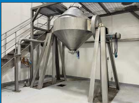
72" Wide x 72" High Single Wall S.S. Conical Blender
