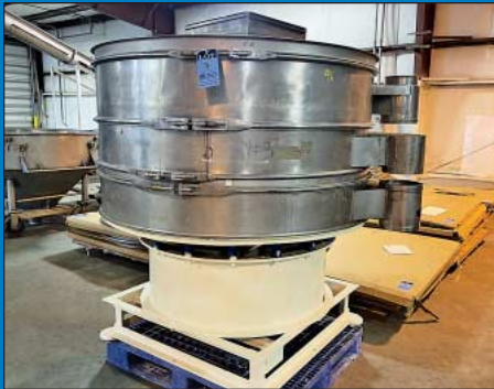
60" Kason Model K-60-2-SS Three-Deck Stainless Screener
