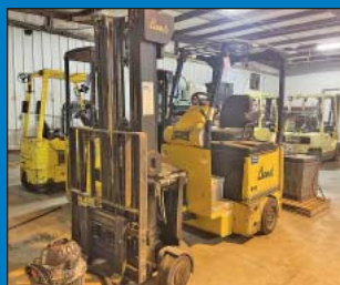
4,000 Lb. Landoll / Bendi Model B-40-1800 Narrow Aisle Articulating Electric Lift Truck
